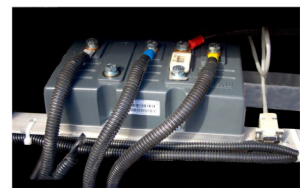
450amp AC Speed Controller
